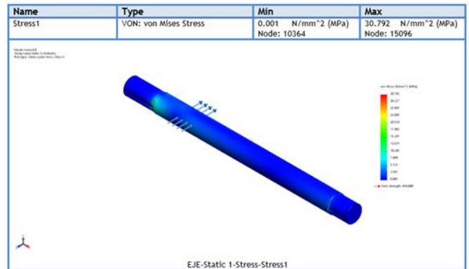
Fig.2: FEA for IS 2062 steel
