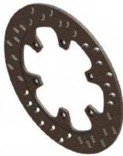
Fig.7: Rendered part of optimized disc brake model
