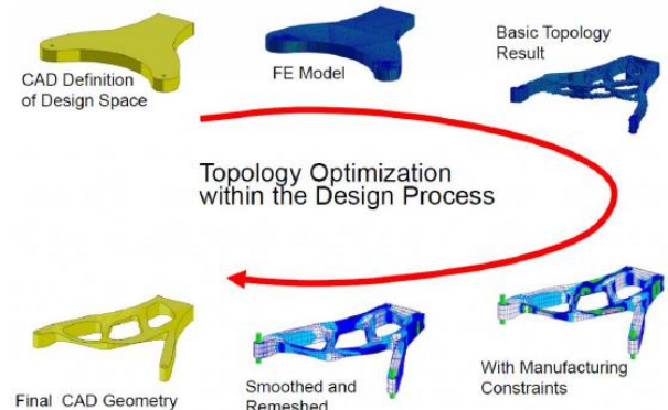
Fig. 1: Stages of topology optimization [5]
