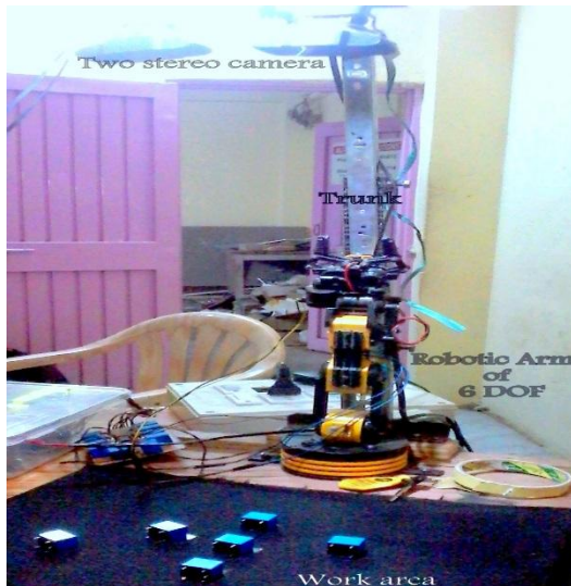
Figure 1: A Pick and Place robo. A six DOF manipulator arm is mounted on a trunk which is fixed on a table. The robot possesses a stereo camera head.
