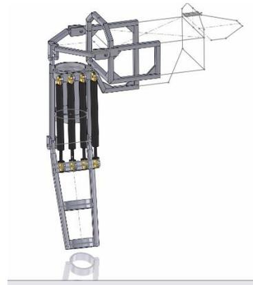
Fig 5.3.3: Screen shot of the SolidWorks CAD model of complete mechanical assembly
