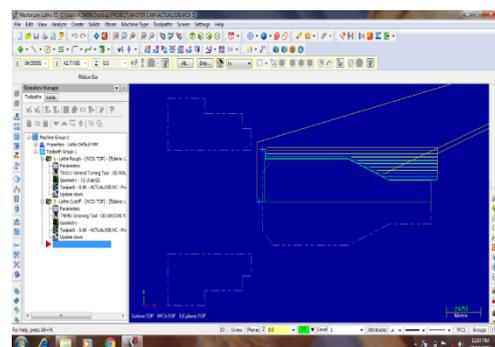
Fig 3.Toolpath of Mastercam
