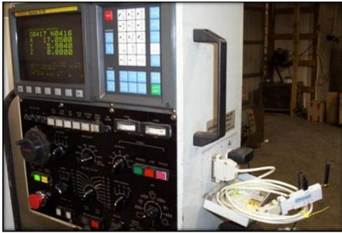
Fig 7: Wireless device (LM058 & LM158) on a Fanuc OM control
